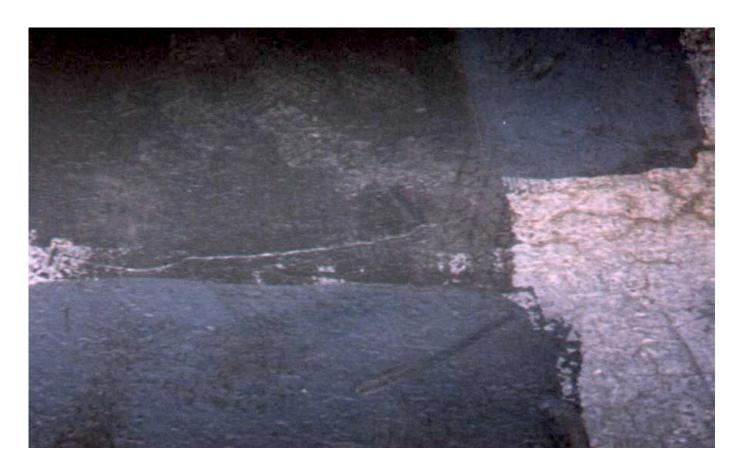
The dark black sample in the upper left is the one with the GSF™; the other two are their old recipe. Notice how strong the color retention is with the GSF™, and the old mix oxidizes as soon as water hits it. All of these samples were put down on the same day.
